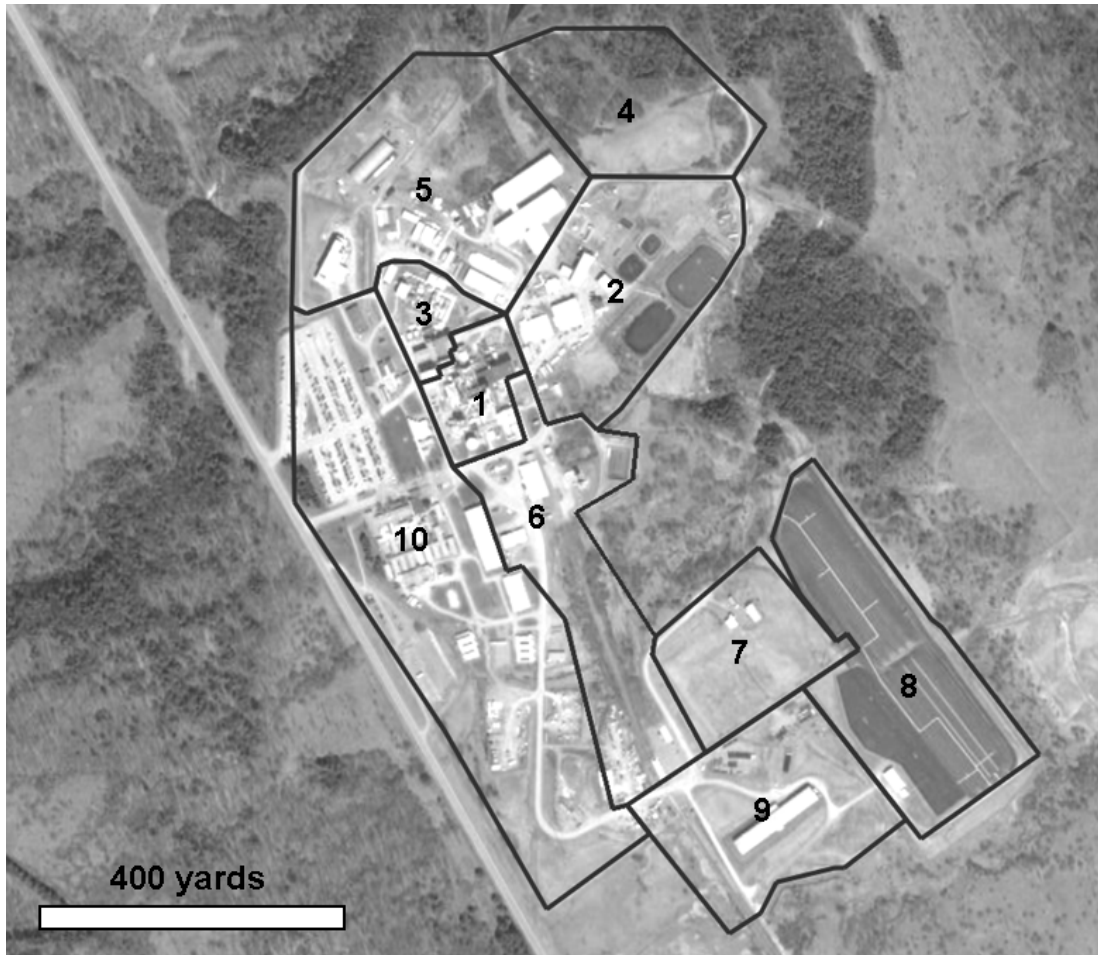
Figure 3.1 Overview of West Valley processing and disposal site. The numbered regions correspond to DOE-labeled waste management areas (WMAs). Primary process building is WMA 1. High-level waste tanks are WMA 3. Groundwater plume extends from WMA 1 through WMAs 2-5. State licensed Disposal Area (SDA) and NRC Disposal Area (NDA) are bounded by WMA 8 and 9, respectively. Rail tracks lead into the south corner of WMA 9. Buttermilk Creek is about 500 yards to the east of WMA 8.
